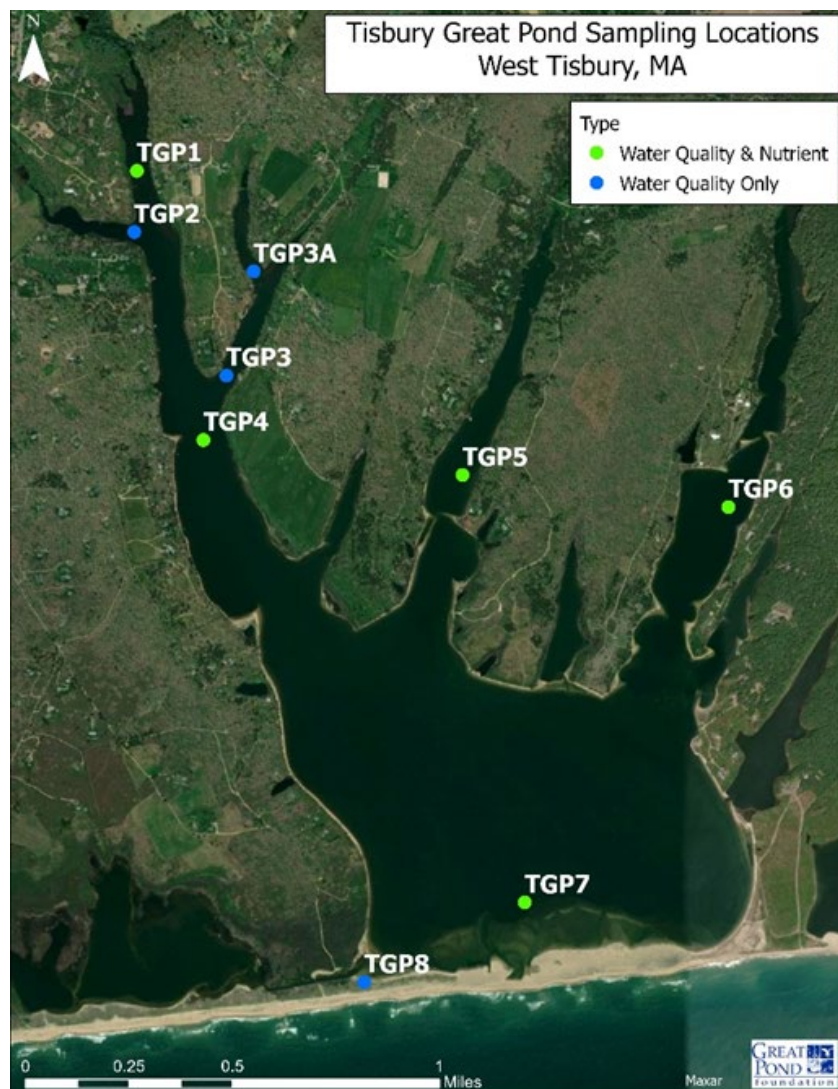
Figure 1. The locations of the 9 monitoring stations used by GPF in 2022 and 2023. Water quality monitoring was conducted at all stations (blue and green), while nutrient sampling was conducted solely at the green stations.
