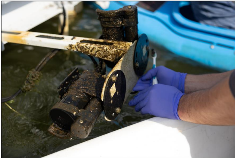
Figure 6. Biofouling on the LG Sonic buoy’s ultrasonic transmitters on 9/23/25. Photo credit: Shenya Leon
