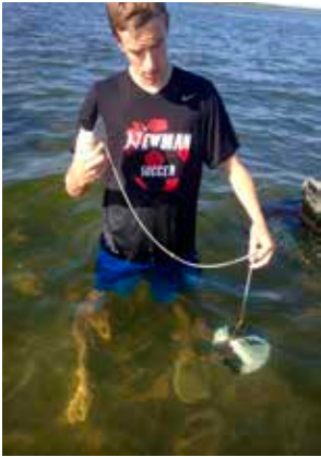
Measuring transparency using a secchi disc
