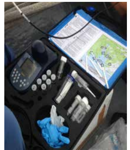
(Right) Photometer on board to measure nutrients present in samples
